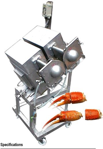
Object material Frozen crab claw Cutter Diamond wheel diameter152x1.5xdiameter25.4 Cutter size 1330/1600m/min Cutter rotating speed AC200V 3-phase 300Wx2 The motor for cutters Cutter edge of a blade interval 15-50mm Dimensions (machine) 680x550x1270mm Weight 90kg Power source 200V 3-phase 50/60Hz
