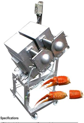
Object material Frozen crab claw Cutter Diamond wheel diameter152x1.5xdiameter25.4 Cutter size Cutter rotating speed 1330/1600m/min AC200V 3-phase 300Wx2 The motor for cutters 15-50mm Cutter edge of a blade interval 680x550x1270mm Dimensions (machine) Weight 200V 3-phase 50/60Hz Power source
